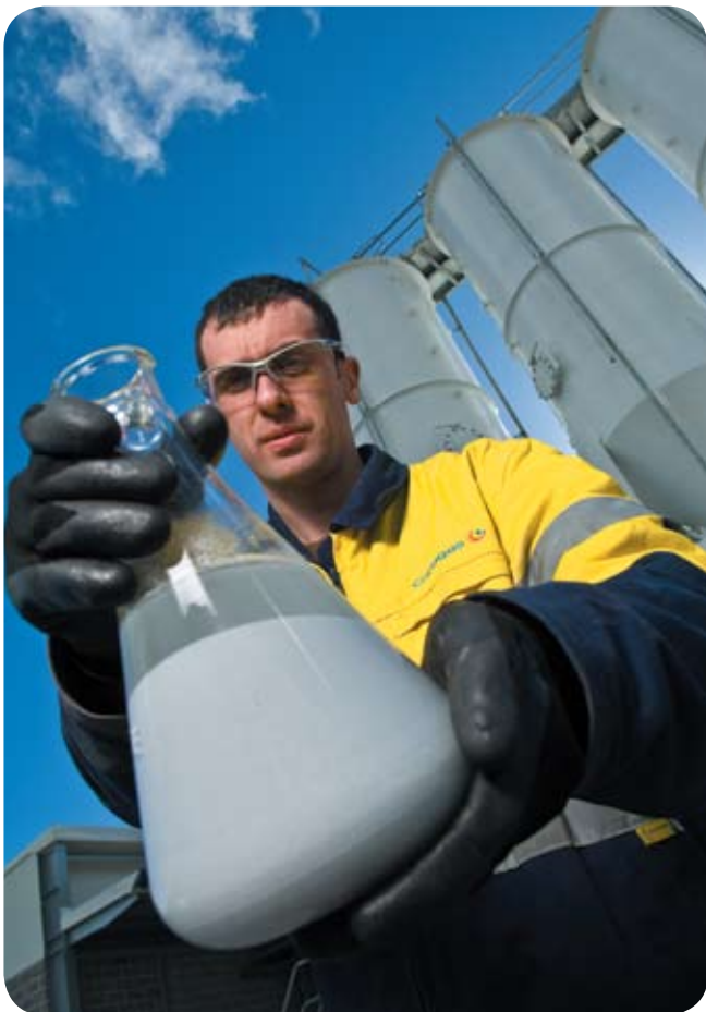
▲ Top: Coregas acetylene filler Daniel Poulos flattening used calcium carbide drums Bottom: Coregas acetylene filler Dylan Raymonds with a beaker of lime slurry, a by-product of acetylene production, which is collected and reused as a soil stabiliser.
