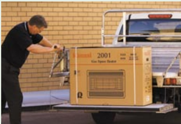
(Left) Compliance Manager Russell Purdy testing a Lyco Loader, a mechanical aid to help reduce manual handling injuries when loading heavy merchandise onto utility vehicles. (Right) Melissa Hewitt using a Lift Aide mechanical device to move heavy stock at the Myaree GasHouse in Western Australia.
