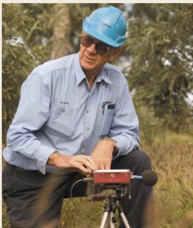
(Right) Senior Engineer Projects Mac Adlam monitoring noise and vibration generated from mine blasts.
