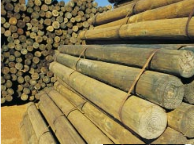
Above Treated pine rounds stacked at Sotico's Mundijong treatment plant. Timber is preserved using a copper, chrome and arsenic (CCA) treatment process.
